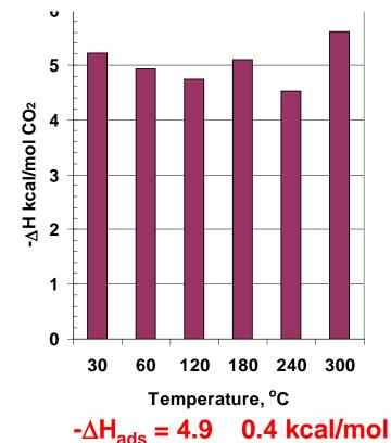
Isosteric heat of adsorption calculations and DSC experiments confirm the low heat of adsorption 8
